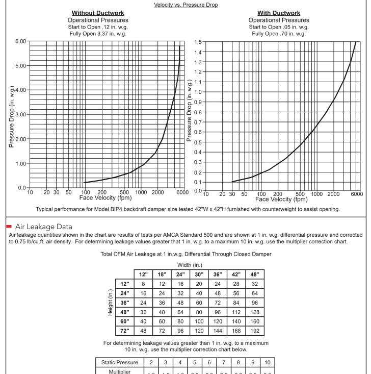
Air leakage ratings are based on AMCA Standard 500 using test set up Fig. 5.4 with damper in the closed position without the aid of a counterweight or other mechanical means to provide closing torque, for a size 42"W x 42"H damper with blade and jamb seals.
